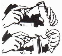
Put thread through needle about  $\frac{1}{2}$  inch. Hold forefinger firmly on reel so it will not turn, and insert needle through material (1). Now notice that you have a short thread end on opposite side of material. Pull this thread out about 18 inches or twice the distance of seam you want to sew.
